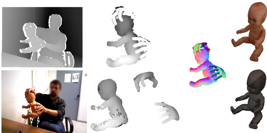
Figure 1: Method overview. Left: input depth and color frames. Middle: Object depth segmented using the fingertip 3D positions. Partially scanned object model and hand models. Right: 3D Rendering of the scene and final scanned model.
