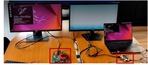
Fig. 5. Use case demo setup. On the left the Kria KV260 board and on the right the Coral TPU Board.
