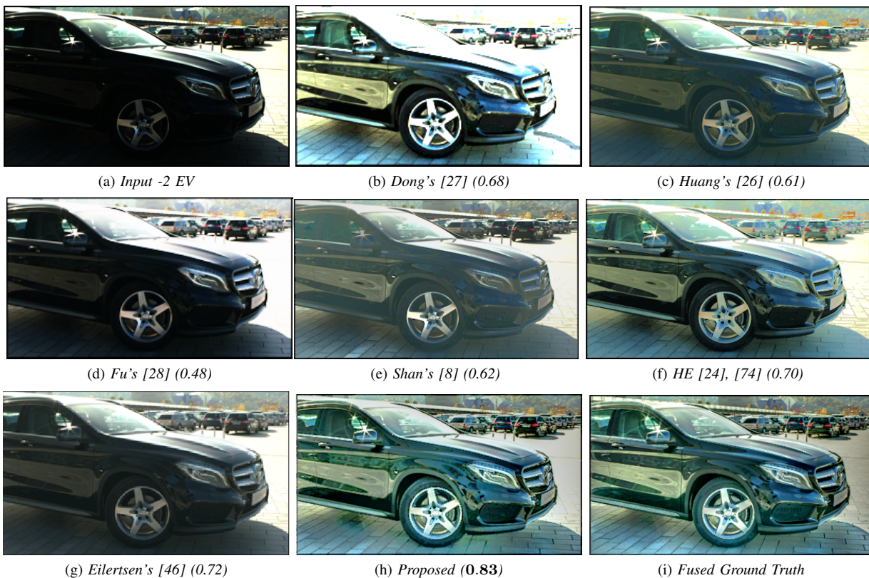
Fig. 11: Car Sequence: Comparison with other state-of-the-art approaches. Unlike the other methods, our system reconstructs successfully both the car's wheel and the region below the car, preserving the background details and providing a smooth, well-enhanced visual result.
