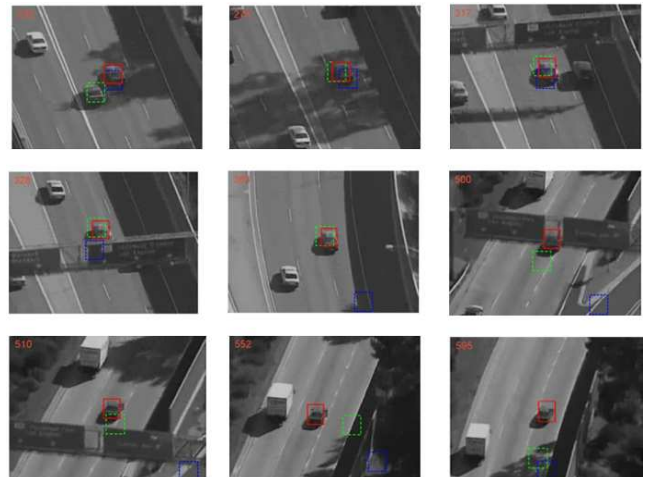
Figure 11: "Car chasing" Sequence. A car is tracked while moving at high speed close to other similarly looking cars and suffering occlusions by the traffic signs.
