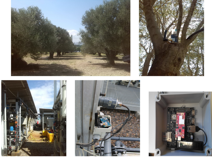
Fig. 8. The experimental deployments at the rural (top) and industrial environments (bottom), and the hardware of node S (bottom right).
