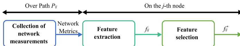
Fig. 3. The three-step procedure for enabling feature selection over multi-hop WSN topologies.
