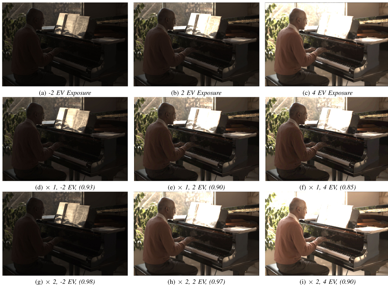
Fig. 6. Double vs. Single Input Scenario. First row: Ground-truth images acquired at -2 , 2 , and 4 EV, respectively. Second row: Reconstructed frames from a single exposure at -4 EV. Third row: Reconstruction from two exposures at -4 EV and 0 EV. We observe that both input cases approximate with high efficiency the ground truth bracketed sequence.
