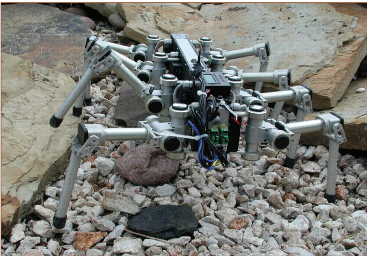
Figure 5. Scorpion robot. The 60-cm, 9.5-kg robot integrates a robust network for navigational and other rules of learning (photo courtesy of Fraunhofer AIS).
