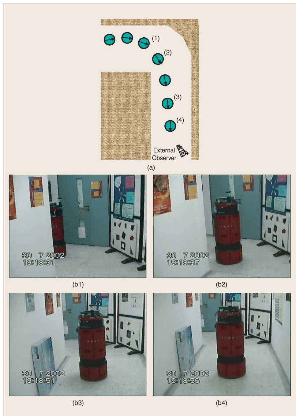
Figure 7. Centering behavior in a T-shaped corridor. Letter captions in (b) roughly correspond to the enumeration of robot positions in (a).
