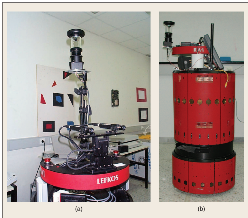
Figure 3. The mobile robot with a panoramic camera mounted on it. (a) The panoramic camera is centered on the robot's axis of rotation. (b) The panoramic camera is displaced significantly from the robot's axis of rotation.
