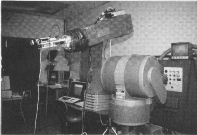
Figure 8. An American Merlin robot arm equipped with TV camera (tracker)
