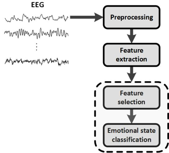
Figure 2. System's submodules workflow
