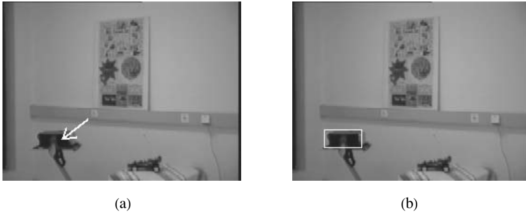
Figure 8: Scene viewed by the camera mounted on TALOS; (a) user selection, (b) constructed template.
