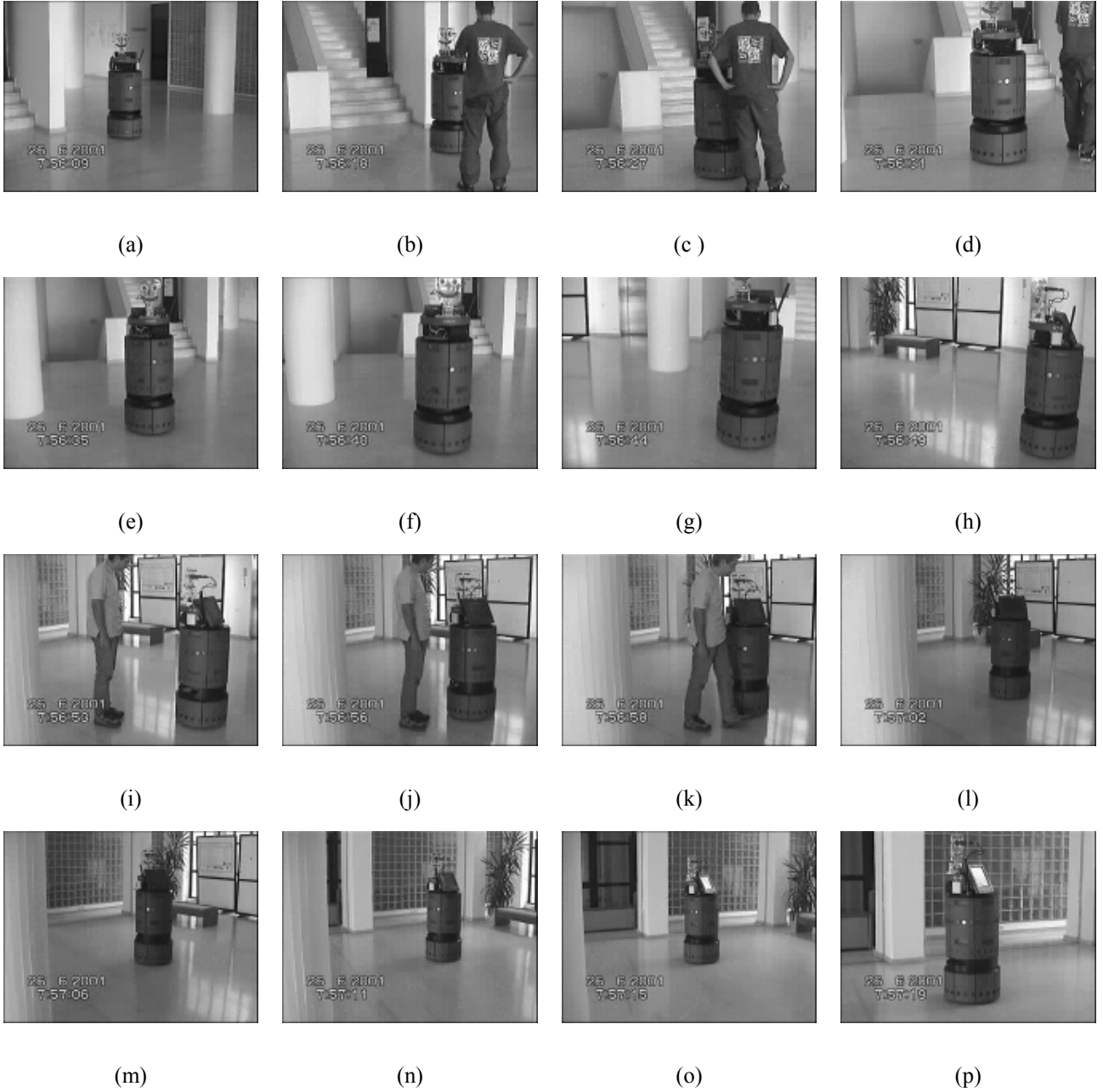
Figure 7: Snapshots from a navigation session. The maneuvers that the robot performs in order to avoid moving obstacles in space can be observed in this experiment.
