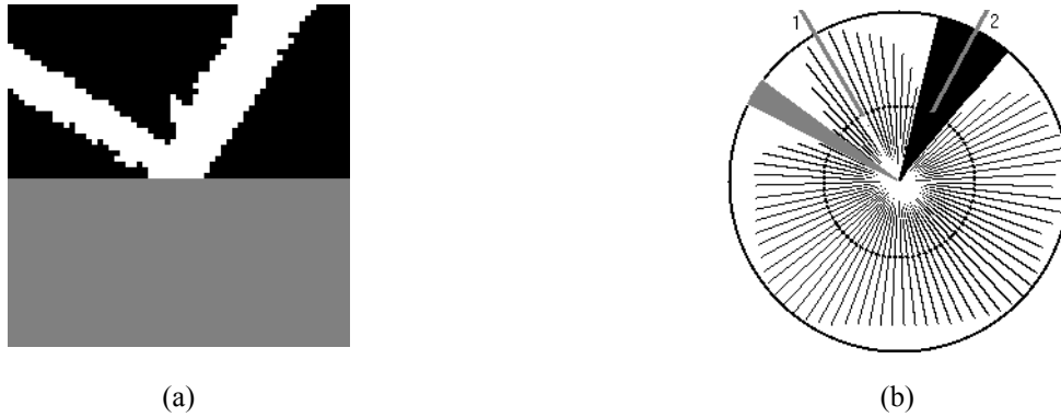
Figure 3: (a) A sample 2D grid-based local map computed from laser readings. White color corresponds to free space, black color corresponds to obstacles and gray color corresponds to lack of information. (b) The vector histogram created from Fig 5(a). Light gray sector defines a non-safe (narrow) space and the dark gray sector defines a safe (wide) space. Although the target direction is along line 1, PYTHEAS will follow the direction along line 2.
