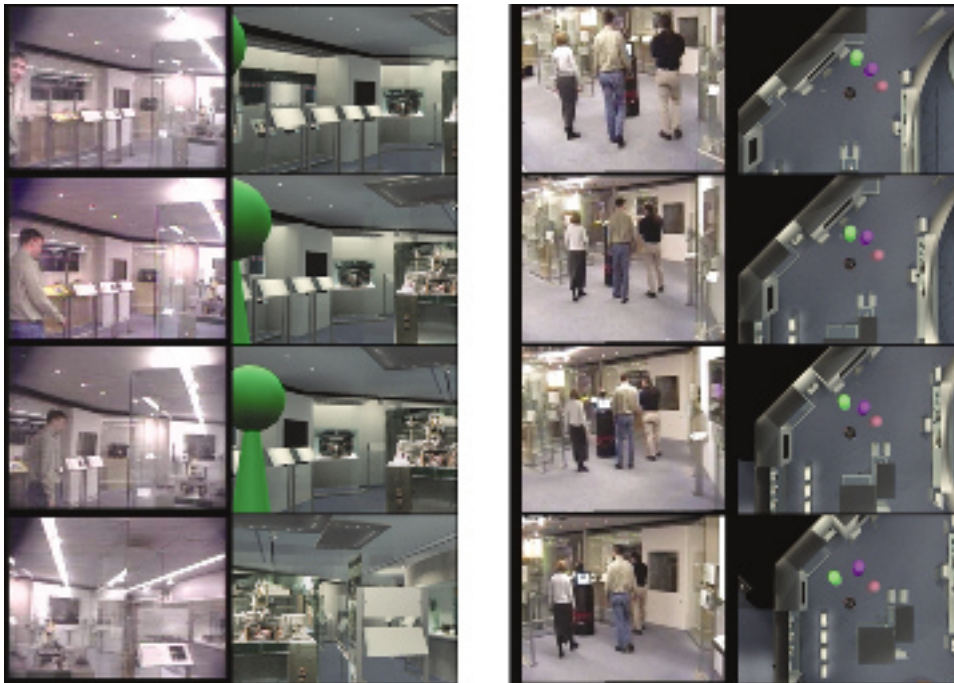
Figure 12. The enhanced 3D visualization allows arbitrary view-points. The left sequence shows the real and the virtual view through the robot's cameras. The right images show the robot guiding three people through the museum and a bird's eye view of the scene.
