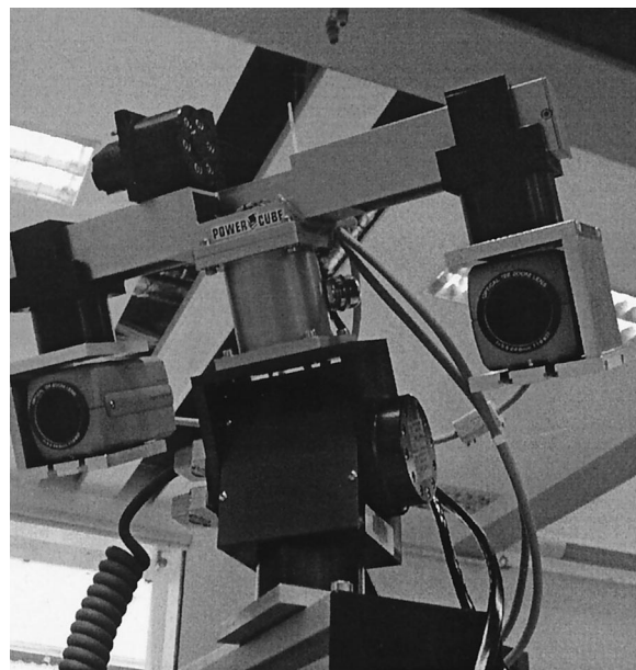
Fig. 1. Stereoscopic head (courtesy of Profactor GmbH) that is used to acquire stereo image pairs that are fed to the SCRT system.
