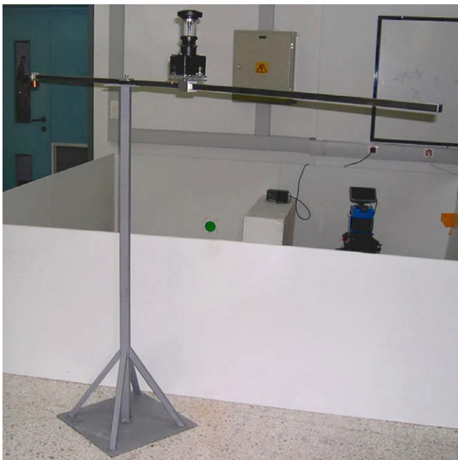
Fig. 3. Imaging setup used for the experiments of Sections 5.1–5.3. The central catadioptric camera is attached to a rotating rigid rod, mounted horizontally on the vertical pole.
