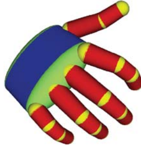
Fig. 1: Hand model with colored parts. Each color denotes a different type of geometric primitive (blue for elliptic cylinders, green for ellipsoids, yellow for spheres and red for cones).
