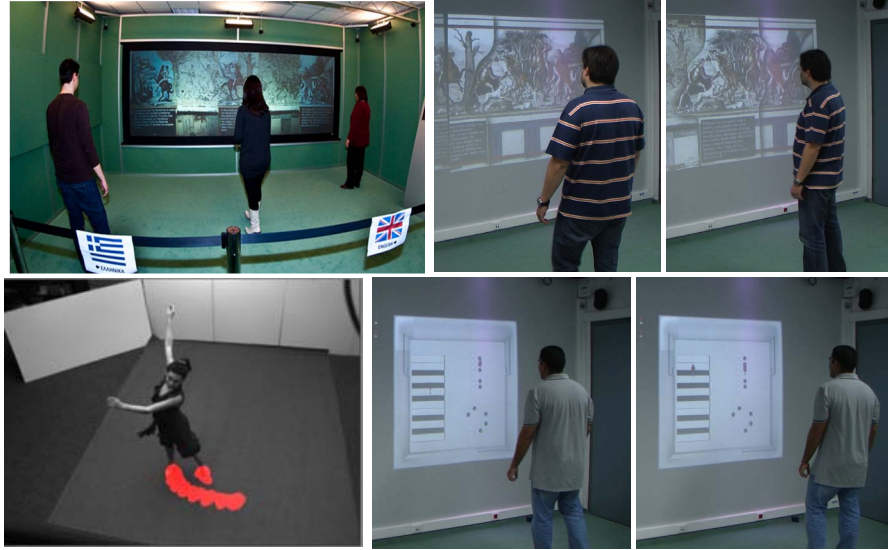
Fig. 4. Pilot applications. Top: The display is updated based on the location and walk-through trajectories of visitors. Bottom-left: footprint extraction; obtained footprints over 20 frames are shown superimposed. Bottom-right: the interactive game’s interface is projected on the wall providing visual feedback to the users, as they play music by stepping in appropriate spots.
