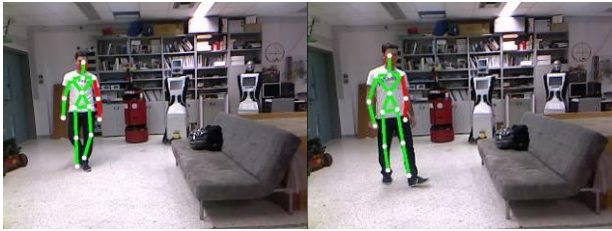
Figure 7: Illustration of 3D skeleton tracking and pose estimation results for two RGB-D data frames. The human body is being tracked with respect to the 3D skeleton model and body poses are estimated based on the acquired depth data for each frame. Only the body limbs and joints are drawn in these sample colored images.
