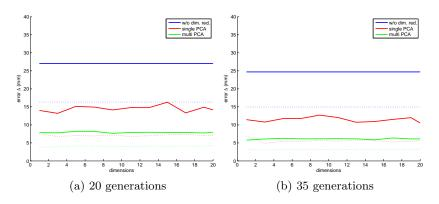
Fig. 4: The error  $\Delta$  for the the 3 algorithms with respect to the number of PCA dimensions and the number of particles: 16 particles drawn as solid line, 64 particles drawn as dotted line. PSO generations are (a) 20 and (b) 35.
