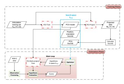
Fig. 1: Graphical illustration of the proposed methodology. At training phase, the reduced dimensionality search space  $S_{7+M}$  is created. At estimation phase, an RGB-D frame is used as input and the best hypothesis is searched for. The enclosed modules at the bottom, form the algorithm's main loop which runs for each generation of the optimizer (PSO).
