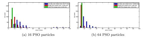
Fig. 5: Histogram of the error  $\Delta$  for all the 3 × 75 estimations per algorithm running for 35 PSO generations with (a) 16 PSO particles and (b) 64 PSO particles. Single-PCA and multi-PCA algorithms used 3 PCA dimensions.
