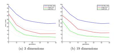
Fig. 3: Error  $\Delta$  with respect to the number of PSO generations and particles: solid line for 16 particles, dotted line for 64 particles. PCA algorithms ran in (a) 3 PCA dimensions and (b) 19 PCA dimensions.
