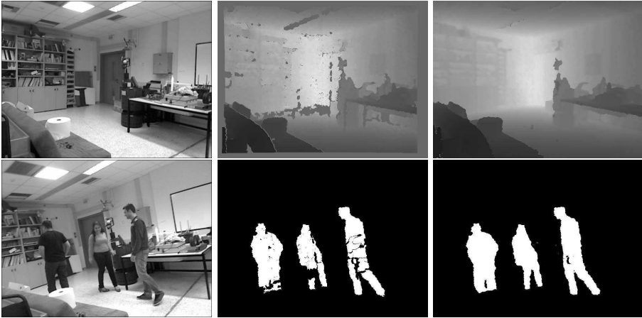
Fig. 4. Top: Background model. I^0 (left). H at time t = 0 ; magenta pixels indicate no depth measurement (middle). H after 1557 frames (right). Bottom: Foreground detection. I (left), result without (middle) and with (right) background history.
