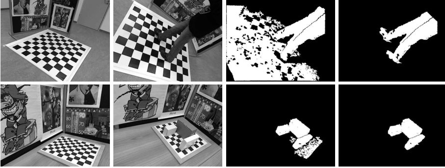
Fig. 3. Comparison of foreground detection methods. Left to right: I^0 , I , and corresponding foreground detection for INIT, and GEN.
