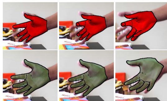
Figure 7. Top row: applying the approach of [27] on the depth maps produced by the ZED camera fails immediately (tracking result in red). Bottom row: the proposed method tracks correctly the hand (tracking result in green). From left to right: frames 1 (initialization), 2 and 15.
