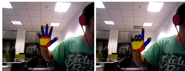
Figure 1: Indicative hand tracker output overlaid over the RGB feed of an RGBD camera source.
