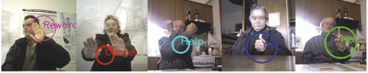
FIGURE 11: Snapshots of Hobbit users performing gestures during lab trials. The recognition results are superimposed as text and a circle on the images indicating the location and the name of the recognized gesture (taken from [19]).
