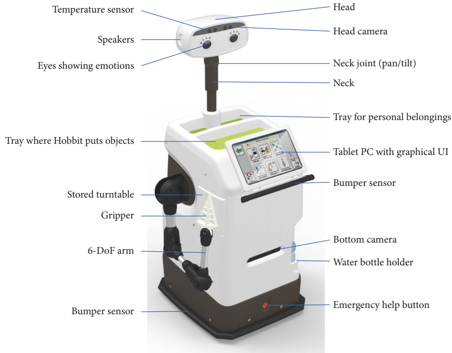
FIGURE 2: Hardware setup of the Hobbit platform.
