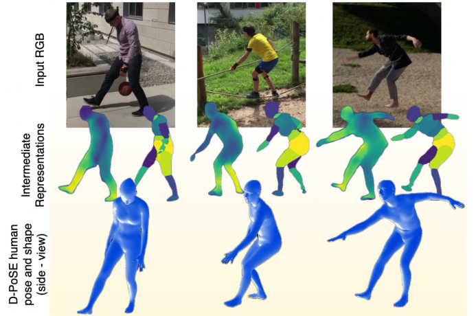
Fig. 1. D-PoSE, the proposed 3D human Pose and Shape Estimation method, receives a single RGB image as input (top), produces intermediate depth and part segmentation representations (middle-left and middle-right, respectively) so as to deliver the 3D pose and shape of the imaged person (bottom, side-view of the mesh for visualization purposes). Despite entailing a small fraction of the parameters of current models, D-PoSE outperforms the current state of the art in 3D pose and shape estimation accuracy in the major relevant datasets (3DPW, EMDB).
