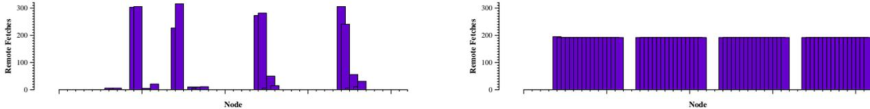
Fig. 7. Distribution of page faults, by processor, in FFTst before (left) and after (right) balancing. (4 nodes, 16 processors per node.)
