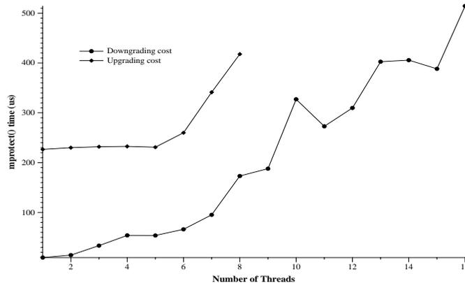
Fig. 3. Average *mprotect* cost for both upgrading and downgrading single pages. Threads in this experiment are competing with each other; although they *mprotect* different pages, they belong to the same share group. This results in TLB invalidations for all processes, as well as contention in kernel data structures.
