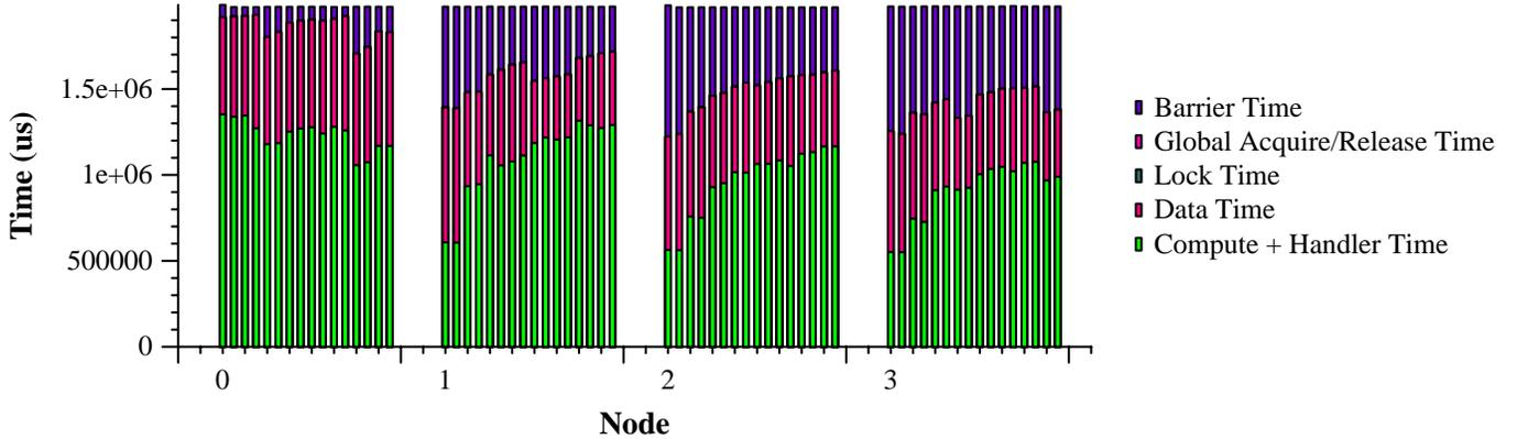
Fig. 6. Breakdown of protocol overhead in FFTst, after balancing. (16 processors per node.)
