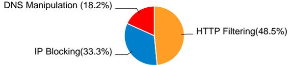
Figure 2: Percentage breakup of the layer at which the filtering was detected during CensMon's evaluation period.
