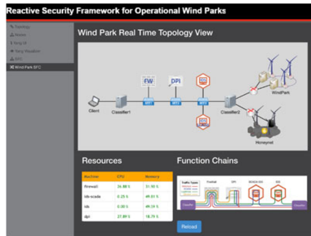
FIGURE 5 Graphical user interface for real-time monitoring of the operation of the reactive security framework on the ODL controller. DPI, deep packet inspection; FW, Firewall; IDS, intrusion detection system; SCADA, supervisory control and data acquisition; SFF, service function forwarder
