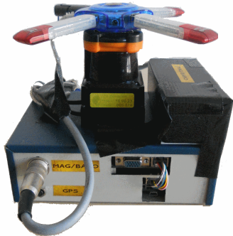
Fig. 1. The handheld laser-scanner hardware comprising a low-cost MEMS Inertial Measurement Unit (IMU), an UTM-30LX LIDAR system and four consumer WiFi cards.
