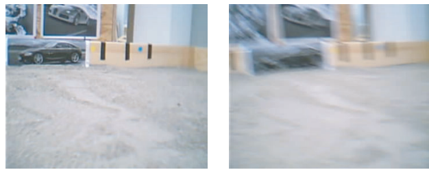
Fig. 6. Two images acquired with the on-board camera and demonstrating the blurring effect caused by the fast head yaw during undulatory movements of the robot. The image on the left has been acquired at the limit of the head yaw, when the lateral velocity is instantaneously zero, and is therefore significantly sharper.
