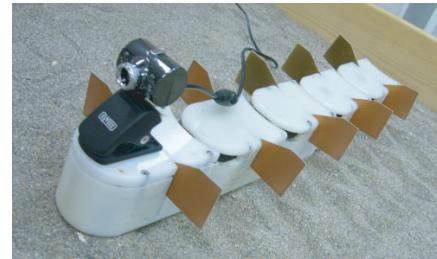
Fig. 1. The Nereisbot undulatory robotic prototype, with an on-board camera mounted on its head link.
