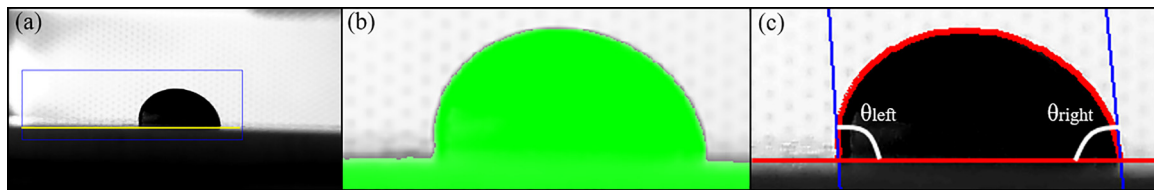
Fig. 2. Side view processing overview. (a) ROI (blue) and horizon (yellow) definition (b) image segmentation (c) contour extraction (red), computation of the tangent (blue) and estimation of contact angles in left ( \theta_{Left} ) and right ( \theta_{Right} ) edges of the droplet. (For interpretation of the references to colour in this figure legend, the reader is referred to the web version of this article.).
