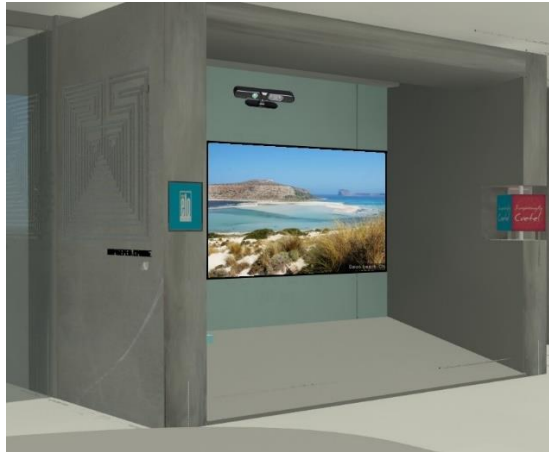
Fig. 1. The setup as designed in a 3D model prototype (a depth sensor is located at the top, a touch screen at the left, an interactive cube at the right and the projection in the middle)
