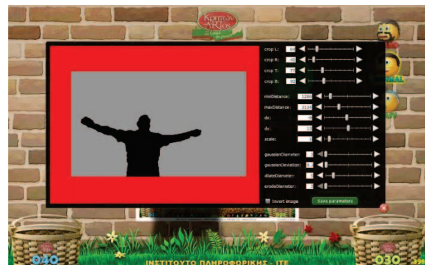
Figure 6. WYSIWYG interface for setting Kinect parameters
