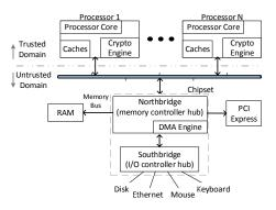
Fig. 1: Data are always encrypted when residing in main memory or moving between the different components of the untrusted domain.
