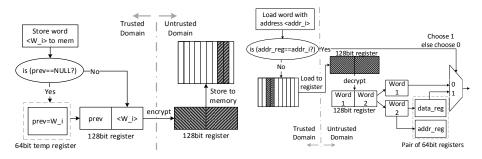
Fig. 2: Subsequent store instructions have Fig. 3: For sequential memory accesses, words encrypted as a bundle in the same the block is decrypted once and the 2nd block and are then stored on main memory. word is retrieved directly from the register instead of re-decrypting the same block.
