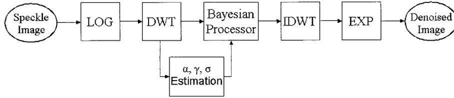
Fig. 1. Block diagram of the proposed multiscale homomorphic Bayesian-based algorithm for speckle suppression. Our proposed novel wavelet coefficient statistical characterization and Bayesian processing modules result in a more accurate ultrasound image reconstruction.
