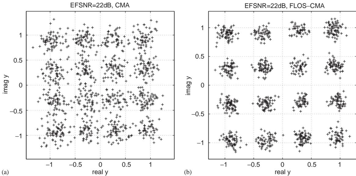
Fig. 6. Signal constellation pattern of equalizer output for the CMA (a) and FLOS-CMA (b). A 16-QAM non-CM input signal is passed through a four-tap channel. Additive  $S\alpha S$  noise is present with  $\alpha = 1.85$  and EFSNR = 22 dB.
