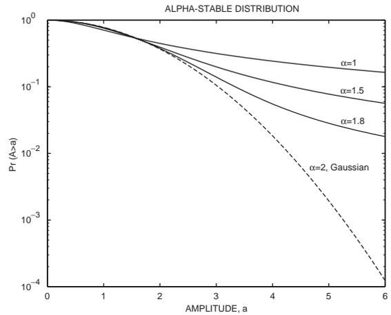
Fig. 1. Symmetric alpha-stable amplitude probability density functions ( $\Pr(A > a)$ ). Dispersion is  $\gamma = 1$  and characteristic exponent is  $\alpha = 1.0, 1.5, 1.8,$  and  $2.0$  (Gaussian).
