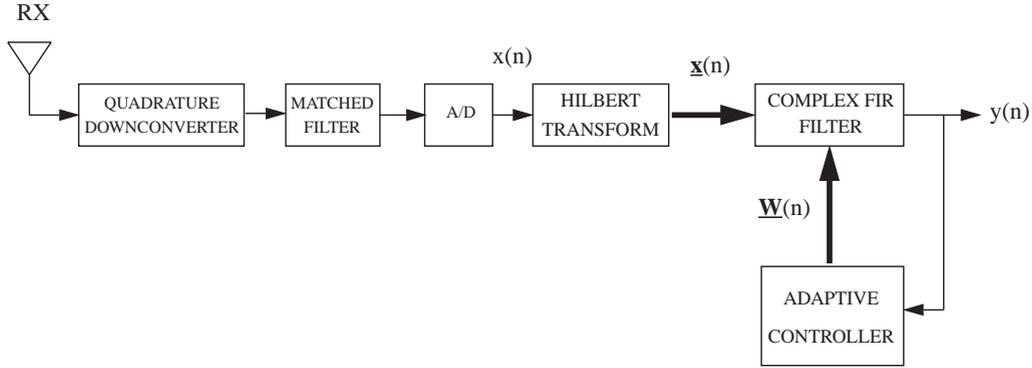
Fig. 2. FIR filter configuration employing the CMA.
