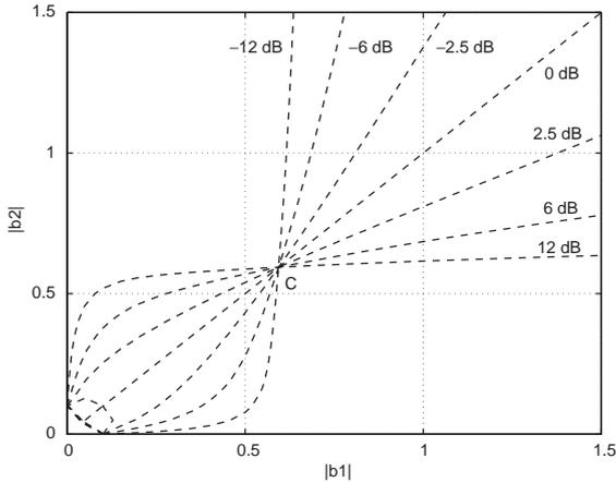
Fig. 4. FLOS-CMA: Lock and capture boundaries as a function of signal-to-interference ratio.
