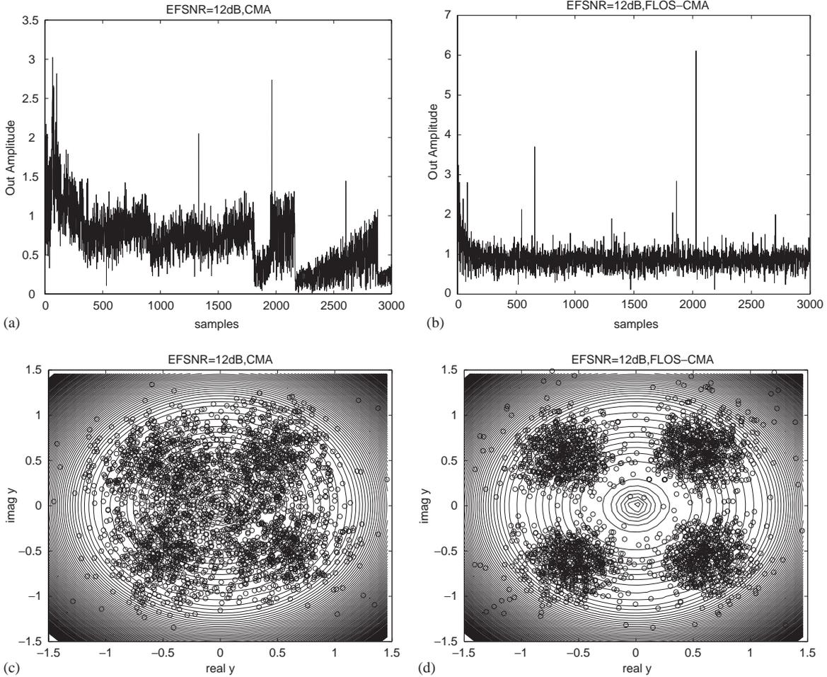
Fig. 5. Amplitude output of the CMA (a) and FLOS-CMA (b). Signal constellation pattern of equalizer output for the CMA (c) and FLOS-CMA (d). A  $\pi/4$  QPSK CM input signal is passed through a two-tap channel. Additive  $S\alpha S$  noise is present with  $\alpha = 1.85$  and EFSNR = 12 dB.
