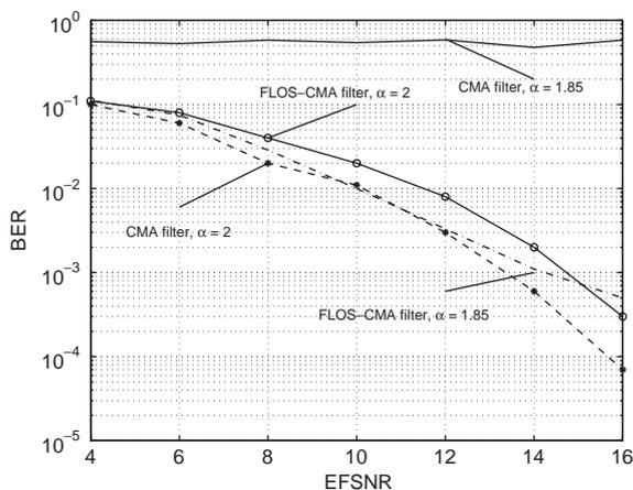
Fig. 7. Bit error rate (BER) versus effective fractional signal-to-noise ratio for the CM and FLOS-CM equalizers in Gaussian ( $\alpha = 2$ ) and  $S\alpha S$  noise with  $\alpha = 1.85$ . The curves correspond to the  $\pi/4$  QPSK input signal and the two-tap channel model.
