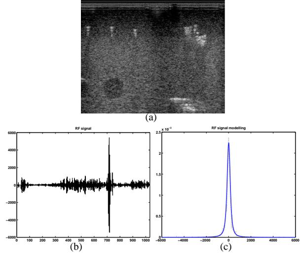
Fig. 1. Example RF signal modelling with  $S\alpha S$  distributions. (a) Original (RF) ultrasound image. (b) An RF signal (one line of the original image). (c)  $S\alpha S$  (continuous line) modelling of RF signal's histogram (dotted line).
