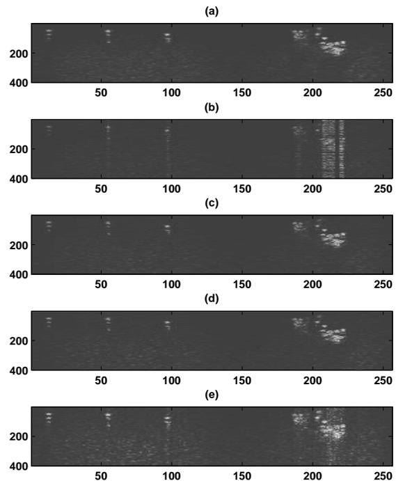
Fig. 2. Comparison of original and reconstructed patches. (a) Original (RF) ultrasound image. Reconstructions with (b)  $\ell_{p_{opt}}$ -norm (c)  $\ell_{\alpha-0.01}$ -norm (d) BP and (e) OMP.
