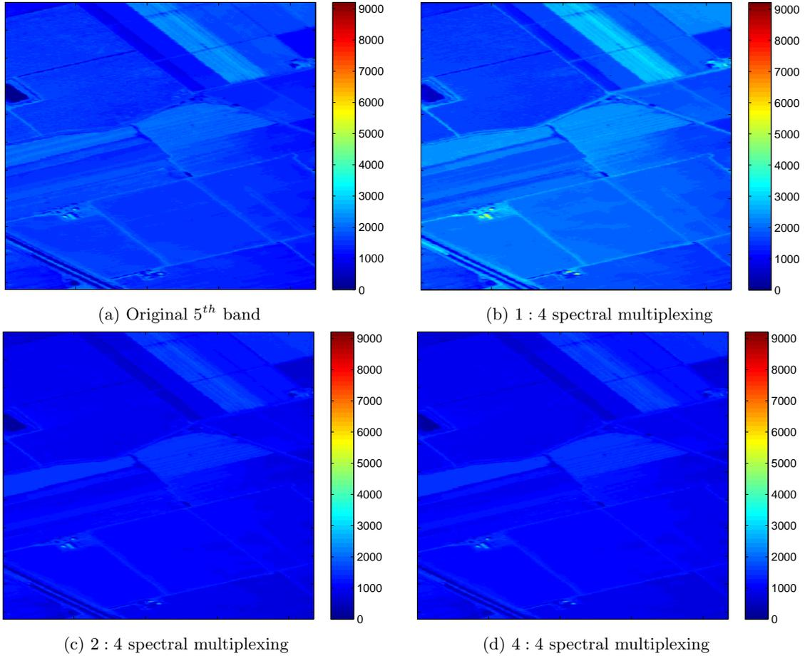
Figure 4: Snapshot HSI recovery of the (a) 5<sup>th</sup> out of 50 bands with (b) 2 : 4, (c) 3 : 4 and (d) 4 : 4 spectral multiplexing. The SNR of the reconstructed images are (b) 15.4 dB, (c) 8.7 dB and (d) 8.8 dB.
