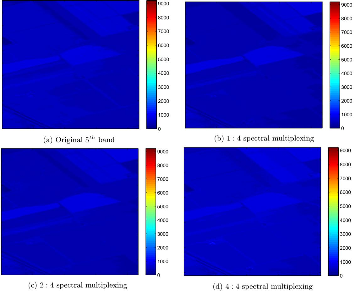
Figure 3: Snapshot HSI recovery of the (a) 5<sup>th</sup> out of 5 bands with (b) 2 : 4, (c) 3 : 4 and (d) 4 : 4 spectral multiplexing. The SNR of the reconstructed images are (b) 18.2 dB, (c) 20.2 dB and (d) 20.5 dB.
