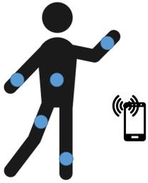
**Figure 1:** The deployment of the wearable sensors (•) for the FORTH-TRACE dataset.
