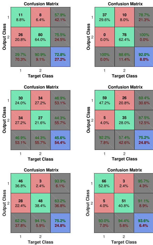
Fig. 4. Confusion matrices for “cycling” (1st row), “dancing flamenco” (2nd row) and “playing the guitar” (3rd row) activities, using motif discovery (left column) and RQA (right column). Green boxes represent true positive (TPR) and true negative (FPR) rates for class 1 (activity) and 2 (non-activity). Red boxes correspond to false positive (FPR) and false negative (FNR) rates. Gray boxes represent the precision and recall percentage (in green) and the error rate (in red). Blue boxes contain the classification accuracy (in green) and expected error rate (in red).
