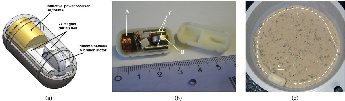
Fig. 3: (a) CAD model of the vibratory capsule. (b) View of the capsule prototype, indicating the 3D coil receiver (A), the coin-shaped vibratory motor (B) and the two permanent magnets (C). (c) Experimental results of the wirelessly powered capsule prototype, propelled by the vibratory motor inside a circular-shaped sand container, which is placed at the center of the external magnetic source (not visible in the picture).
