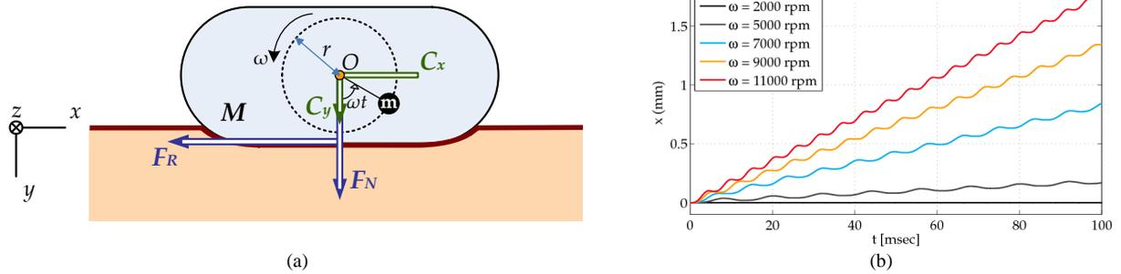
Fig. 2: (a) Mechanical model of the vibratory locomotion system. (b) Simulation results, indicating the capsule's horizontal advancement, as a function of the rotational velocity of the eccentric mass.
