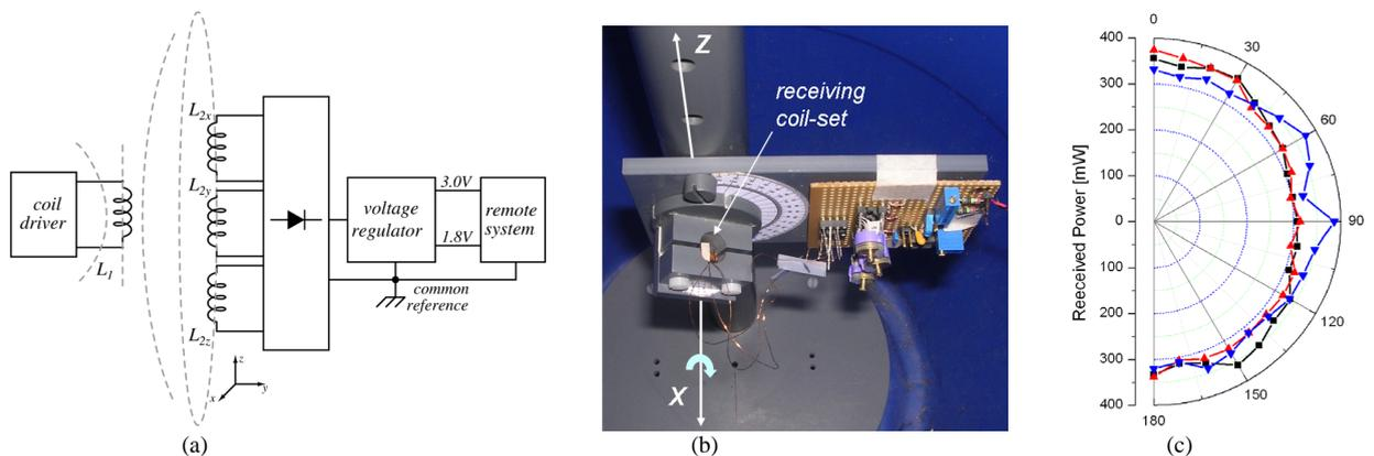
Fig. 1: Block level schematic (a) and characterization of the 9mm ferrite coils (b) and (c). The measurement is relative to a mmf of 68 A-turns. The receiver is placed at the center of  $L_1$ , readings are taken with steps of  $10^\circ$  while performing a  $180^\circ$  rotation.
