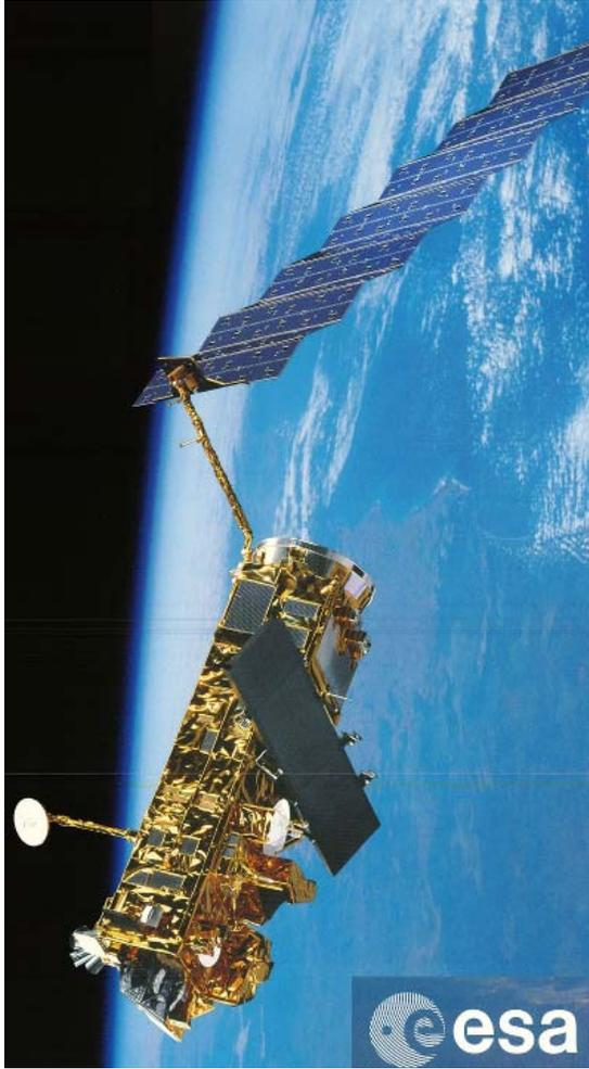
Fig. 1. Visualization of ENVISAT ©ESA, the target debris of e.Deorbit.
