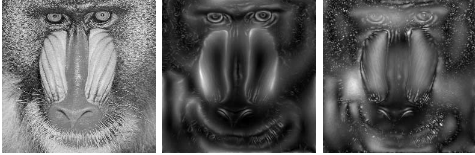
Figure 1: An image (left) and the SSR scale selector response for edges (middle) and blobs (right).
