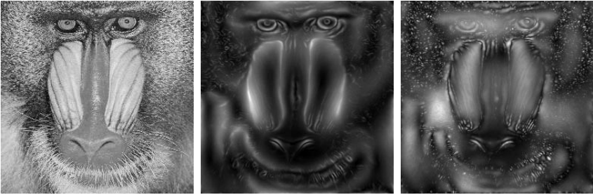
Fig. 1. An image (left) and the SSR scale selector response for edges (middle) and blobs (right).
