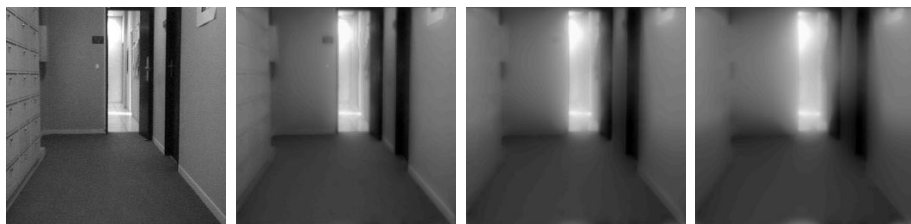
Fig. 6. Image evolution in scale space created by SSR smoothing (from left to right).
