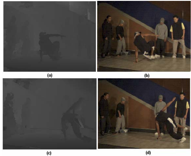
Figure 6: (a),(c) estimated depth maps of the reference images; (b),(d) reference images at different time instants
