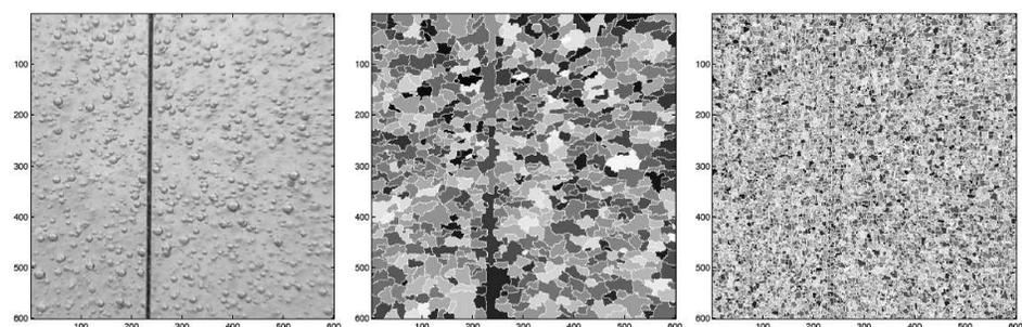
As a result, typical contrast-based segmentation techniques do not suffice for bubble-detection purposes. The images above, show an original image and its watershed segmentation for two different numbers of iterations.
