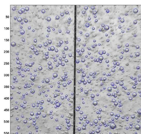
The images above and on the left demonstrate the performance of the proposed method by marking the detected (focused) bubbles. As it can be observed, the method not only discriminates between focused and unfocused bubbles but is robust against bubble overlap, which is typical in dense dispersions.
