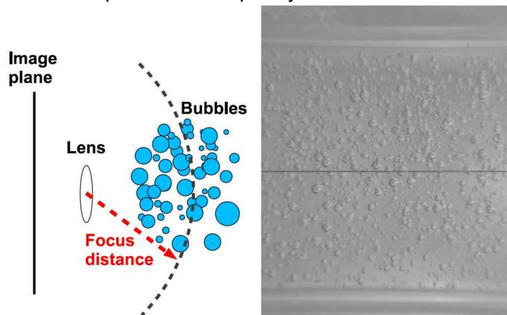
Left: the bubble measurement apparatus; only bubbles at the focus distance will appear focused in the image. Right: an 2560 1920 image obtained from this apparatus.
