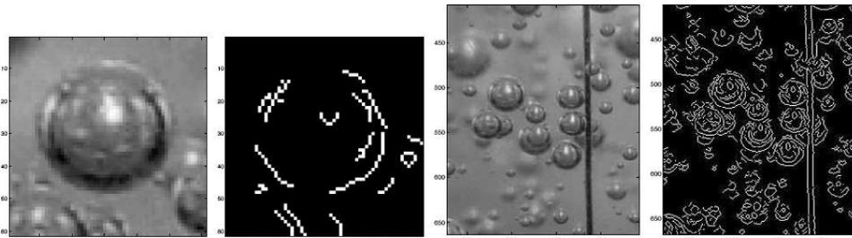
Details of two original and edge images. Reflections, occlusions, shadows, and highlights give rise to complex edge images that are difficult to directly use to estimate bubble shape.
