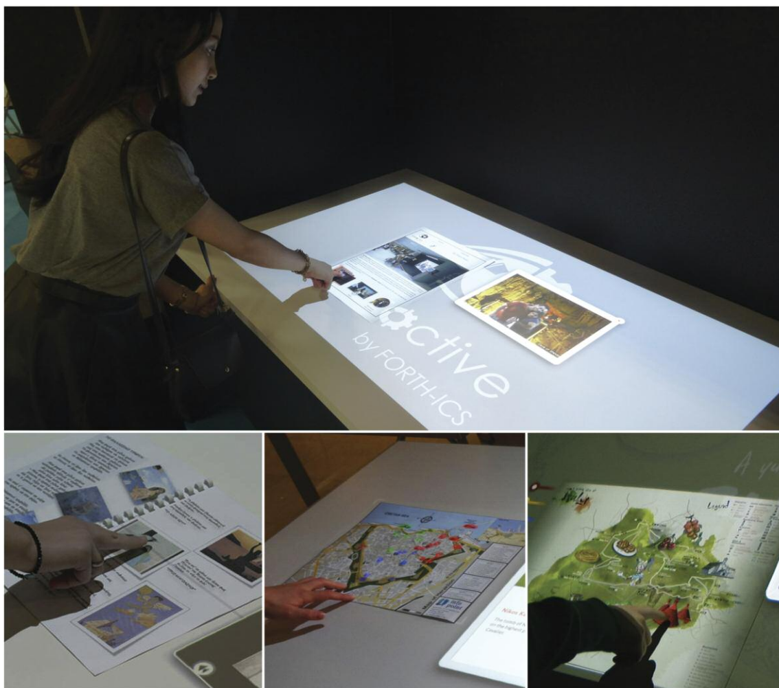
Figure 1: User interaction with augmented printed documents. Main: the system highlights regions of potential user interest; upon user touch, relevant content is augmented, juxtaposed to the document. Thumbnails: multimedia augmentation in a music and poetry book (left), map augmentation providing city tour information on the printed map (middle) and visitor information (right).
